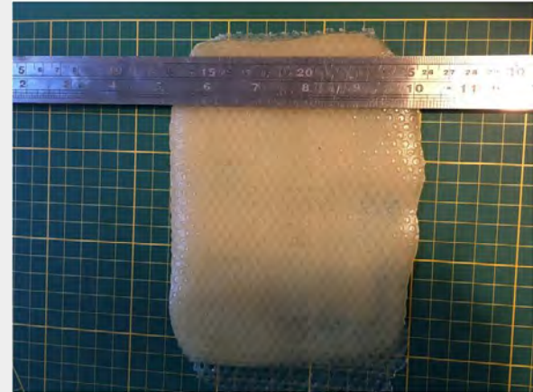
Trimming the - still flexible - slab for further curing, Loes Bogers, 2020
